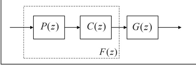
FIGURE 3: Realization of Approximate Non-minimum phase-zero Inversion
