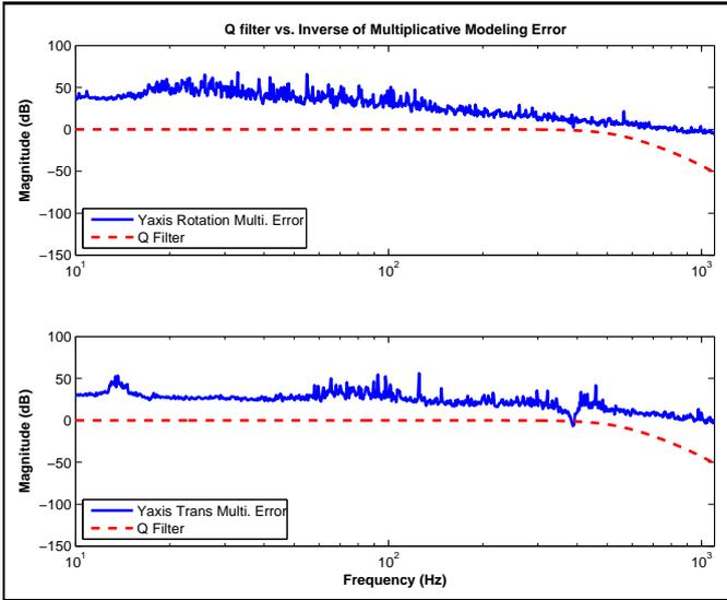
**FIGURE 7:** Magnitude of Q filter vs. Inverse of Multiplicative Modeling Error for Robust Stability of Translational and Rotational Systems
