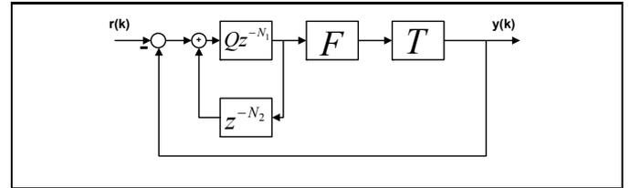
FIGURE 5: Repetitive Control with Feedforward Inversion and Lead controller
