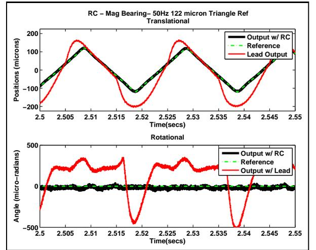
**FIGURE 8:** Tracking Performance Comparison of Lead and Proposed Repetitive Controller
