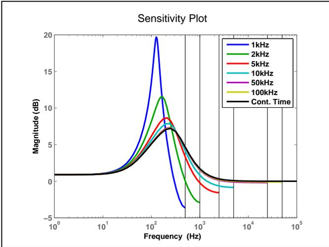
FIGURE 4: Sensitivity Function with different Sampling Rates
