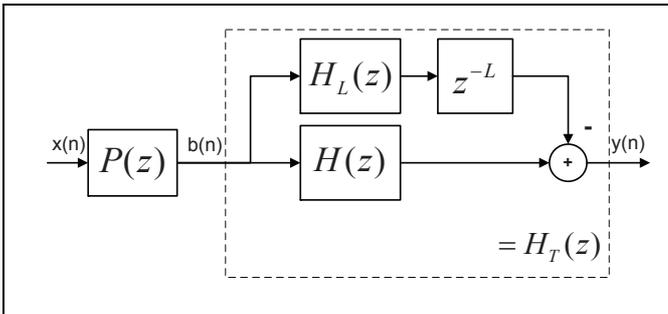
FIGURE 2: Realization of Kurosu's Exact Linear Phase IIR Filter
