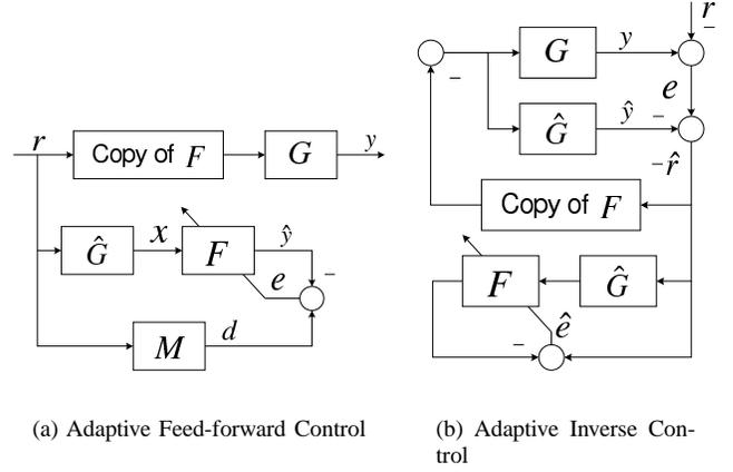
Fig. 3. Adaptive Control Structures for Reference Tracking
