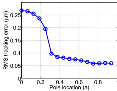
Fig. 9. Root-Mean-Square (RMS) error v.s. pole location  $a$
