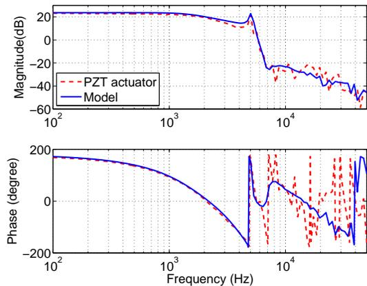
Fig. 4. Frequency Response of PZT actuator and Model
