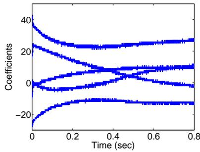
Fig. 8. Coefficients update of Laguerre filters using LMS algorithm
