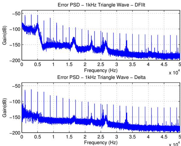
Fig. 10. Error PSD with 1kHz Triangular Wave Reference Tracking.
