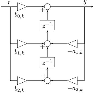
Fig. 5. Direct Form II Transposed Implementation
