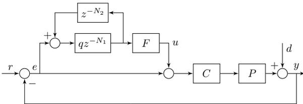
Fig. 8. RC with feed-forward inversion and PI controller.
