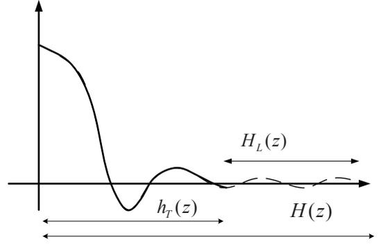
Fig. 1. Truncation of infinite impulse response at  $L^{\text{th}}$  sample.
