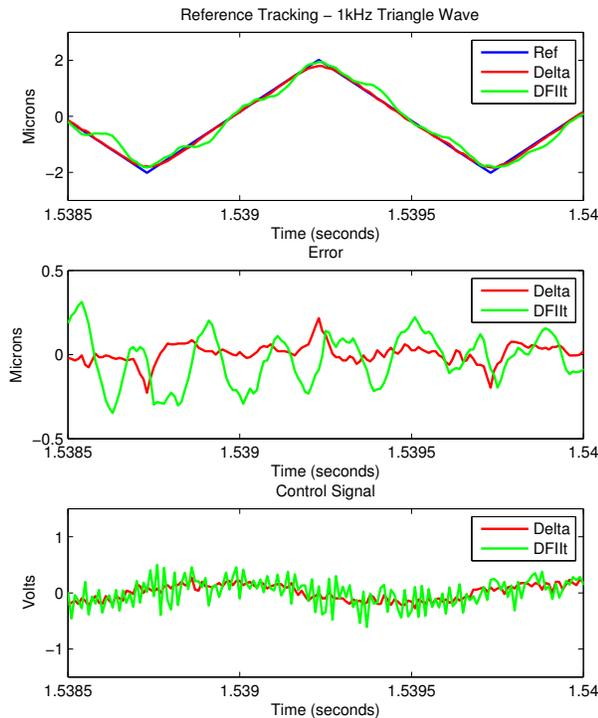
Fig. 9. Reference Tracking and Error of 1kHz Triangular Wave.
