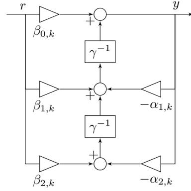
Fig. 6. Direct Form II Transposed Implementation - Delta Operator
