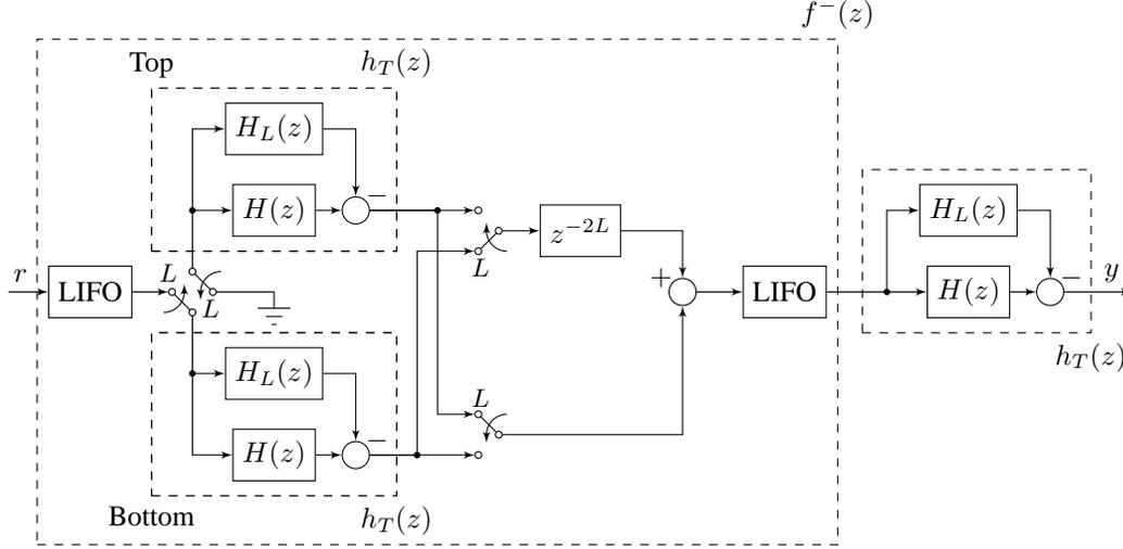
Fig. 2. Kurosu's exact linear phase filter.
